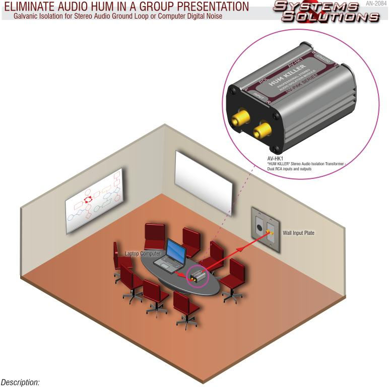
Presentations using a laptop computer face problems of delivering quality audio through an unbalanced connection. Any difference in ground potential between the computer and audio amplifier creates "hum" that becomes part of the presentation audio. In some systems, digital noise from the computer may also add a constant irritating background noise to the audio.
