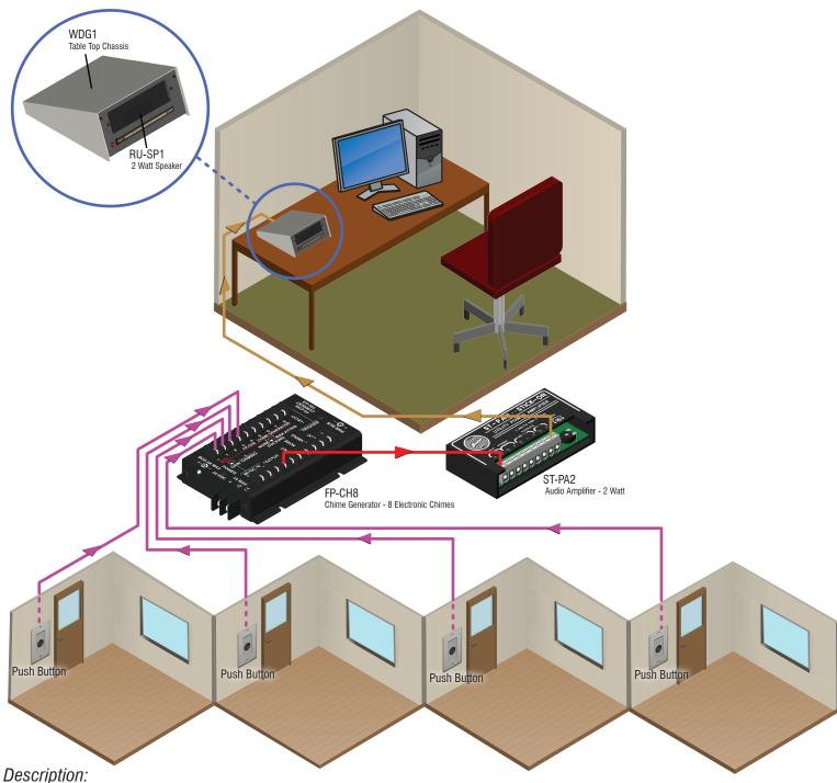
The RDL FP-CH8 Chime Generator is the solution when it is necessary to associate a unique sound with specific events. In this example, four of the eight available chime tones are used. A particular chime identifies which doorbell button is pushed.
