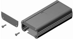
Remove the lower (larger) cover at the left end of the unit using the two screws shown. Connect the wires from the SourceFlex controller as indicated in the connection diagram. Secure cover.
